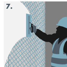
Covering mesh with basecoat.
