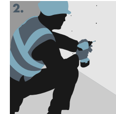
Fixing the boards to the background members.
