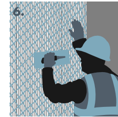
Applying reinforcing mesh.
